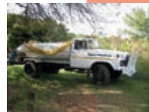
Desludging Equipment (Honey sucking Trucks) Maintenance, Drainage, Suction of Full Ventilated Improved Pits and Septic Tanks.
